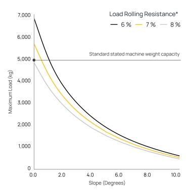
\* Variables that affect rolling resistance include the quality of floor/terrain and the type/condition/quality of castor wheels.
