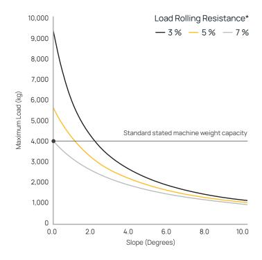
\* Variables that affect rolling resistance include the quality of floor/terrain and the type/condition/quality of castor wheels.
