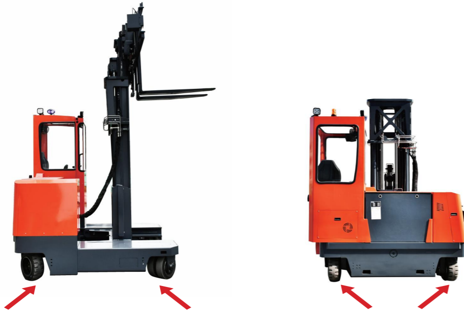
Solid rubber tire Solid rubber tire Dual drive, dual electromagnetic braking
