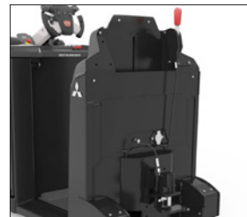
Automatic coupling with ergonomic unlocking handle
