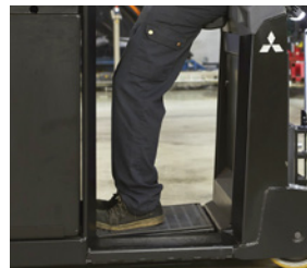
Suspended operator's platform.
