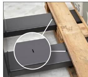
Crossway pallet indication on forks
