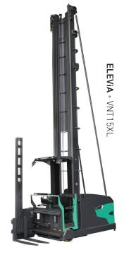
of trucks. The 1.1-1.3 tonne models are available with 48v or 80v electrical systems, while larger models are 80v only.
